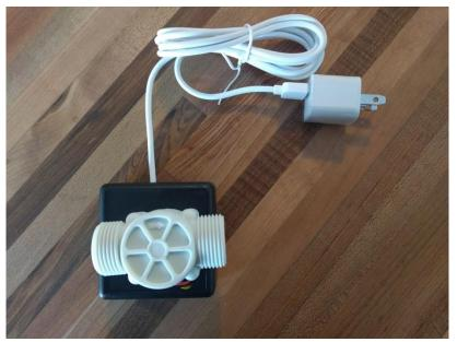
Each water meter is labeled on the underside of the black enclosure with pre-programmed apartment address. On the underside of the white meter connection there is a small white arrow for direction of flow. Be sure to install meter in correct orientation.
