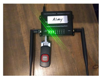
Just plug the router into a wall outlet in a common area, utility room or somewhere as discrete as possible. Some routers will look different. Once powered up check that all lights are lighting up. If you do not have cellular signal on your cell phone chances are the True Submeter modem does not have cellular connection either. (Note: some of our routers look slightly different and are black, have different USB modems and antennas)
