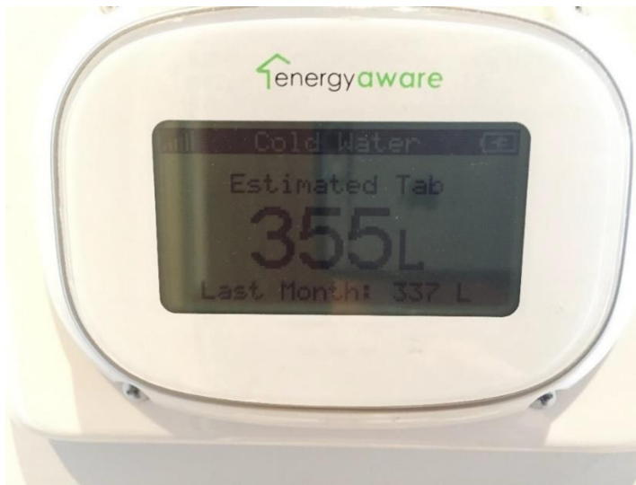
Figure 17. An in-suite monitor that shows the monthly cold water consumption of a unit at Olympic Village (photo courtesy: Andrew Ling).
